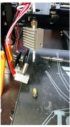
7.Heat up the heatbreak and push the plastic out of the heatbreak or drill it out with a 4mm drill bit
